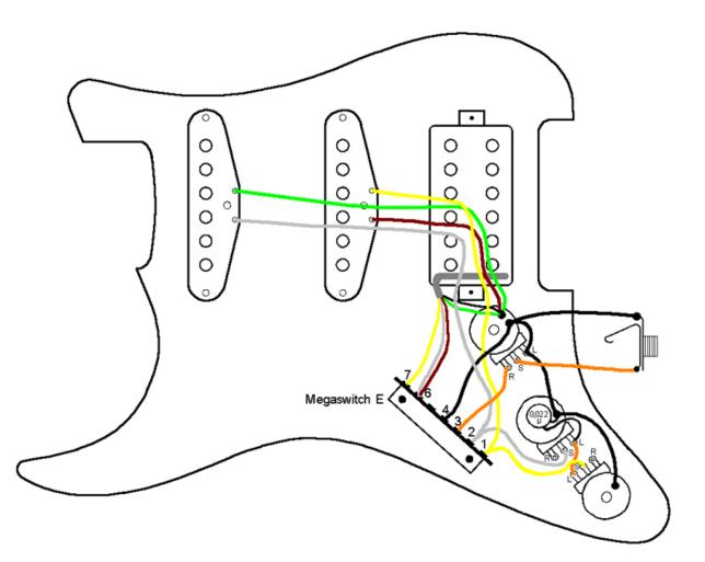
Positions 1 bridge humbucker 2 bridge inner coil and mid parallel 3 bridge outer coil and neck 4 mid and neck parallel 5 neck
