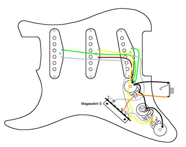
Positions 1 bridge 2 bridge and mid parallel 3 bridge and neck parallel 4 mid and neck parallel 5 neck
