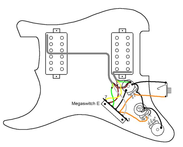
Positions 1 bridge humbucker 2 bridge inner coil 3 outer coils parallel 4 neck outer coil 5 neck humbucker
