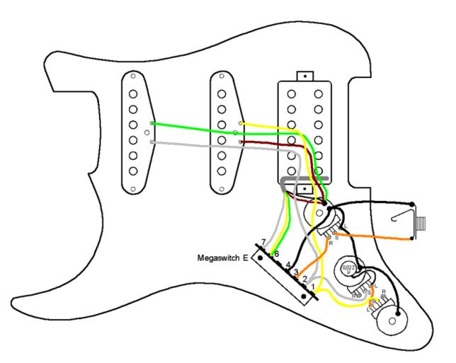
Positions 1 bridge humbucker 2 bridge outer coil and mid parallel 3 bridge inner coil and neck 4 mid and neck parallel 5 neck
