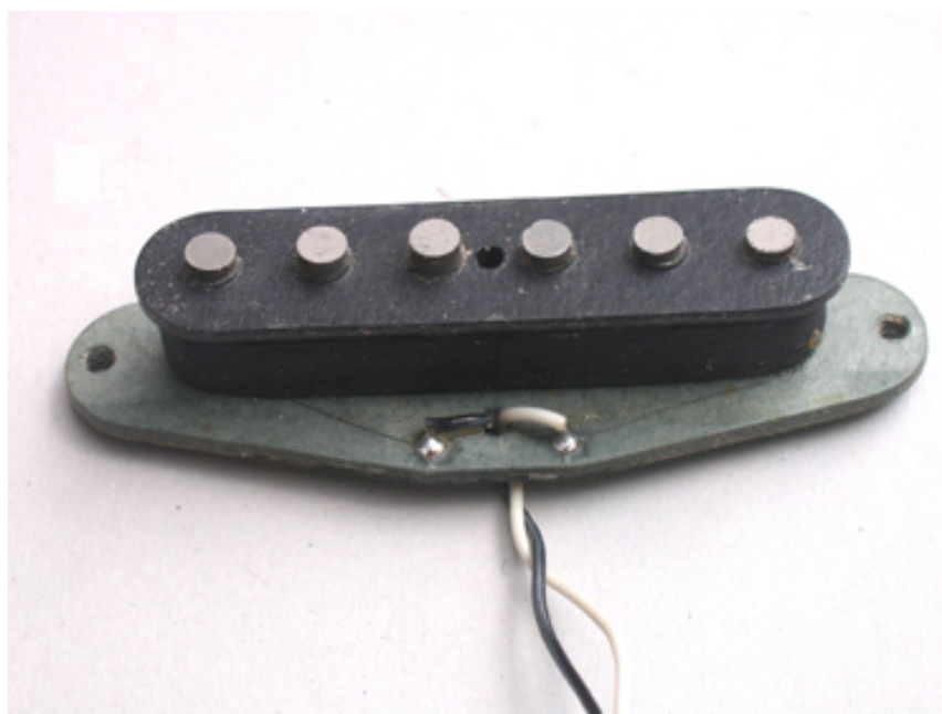
Figura 1. Pickup Stratocaster, intrinsecamente simmetrico
