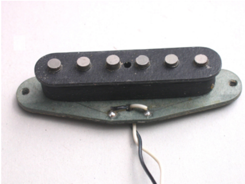
Figure1. Stratocaster pickup (symmetric by nature)
